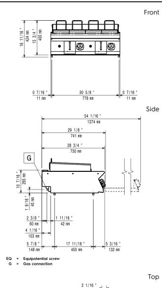
Gas Gas Power: 14 kW Standard gas delivery: Natural Gas Type Option:
